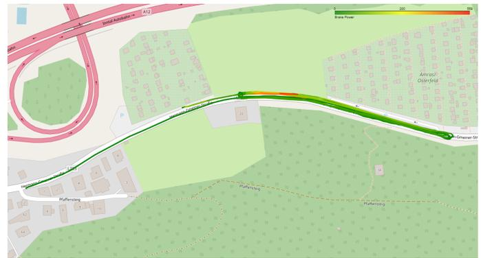
Fig. 3. Spatial Visualization of Brake Power.
