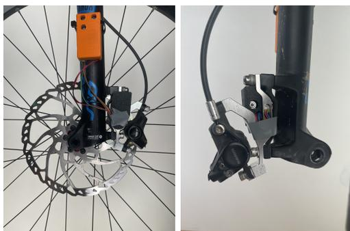
Fig. 2. Left (left) and right (right) views of the installed brake force sensor system, with and without wheel installed.
