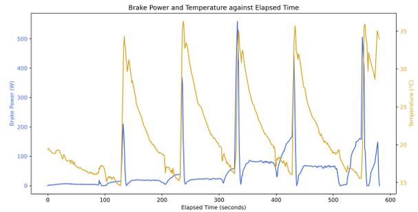
Fig. 7. Brake Power and Temperature against Elapsed Time.
