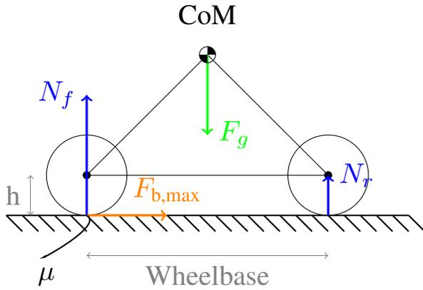
Fig. 1. Diagram illustrating the braking dynamics of a bicycle.
