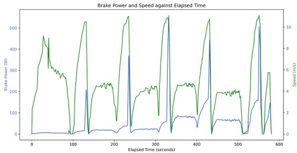
Fig. 5. Brake Power and Speed against Elapsed Time.
